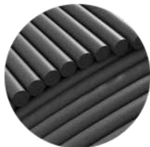
Nylon is a robust and durable artificial fiber traditionally used for strong tyre casings. Nylon threads are less thin than cotton ones, so casings have a lower number of threads per inch. The advantages of nylon casings is that they are strong and durable, extending the wear life of the casing. However, because it is an artificial fiber, it is not as supple as cotton.
