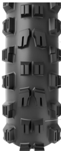
Aggressive tread profile with ample side tread spacing
